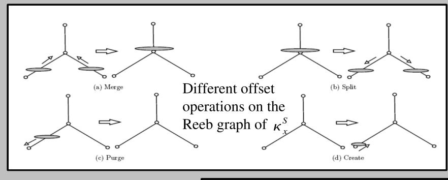
Offset operations used to simplify the Jacobi set. Purge and Merge operations reduce the number of Jacobi set components.
