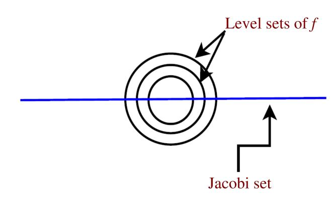
Jacobi set (blue line) for the functions  $f = x^2 + y^2$ and g=x. The Jacobi set of two functions defined on a 2-manifold is the set of points where the gradients of the functions align with each other.
